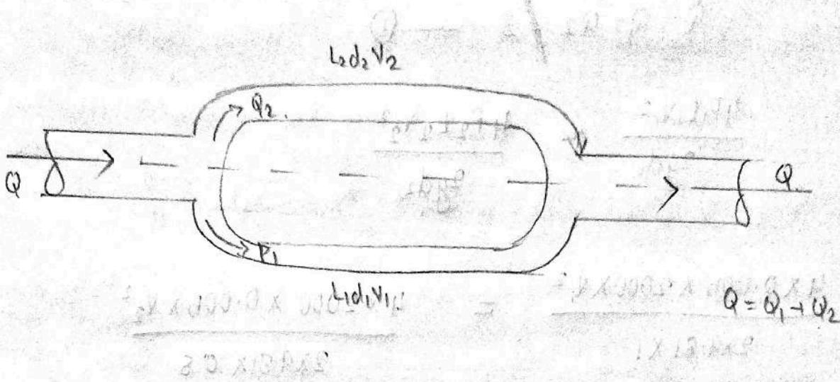
$$\frac{4f_1L_1V_1^2}{d_1x_2g} = \frac{4f_2L_2V_2^2}{2gd_2}$$
