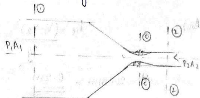
$$② h_e = \frac{(V_1 - V_2)^2}{2g}$$
